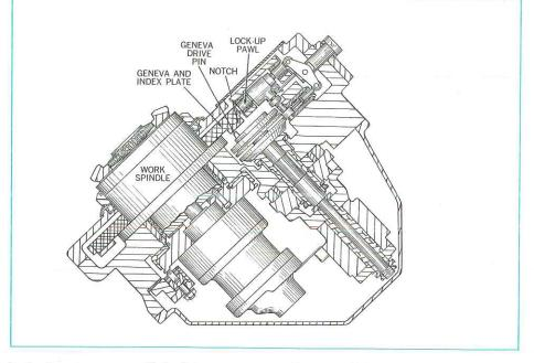
Indexing is accomplished by an entirely new mechanical-hydraulic system to assure a faster and more accurate index.
