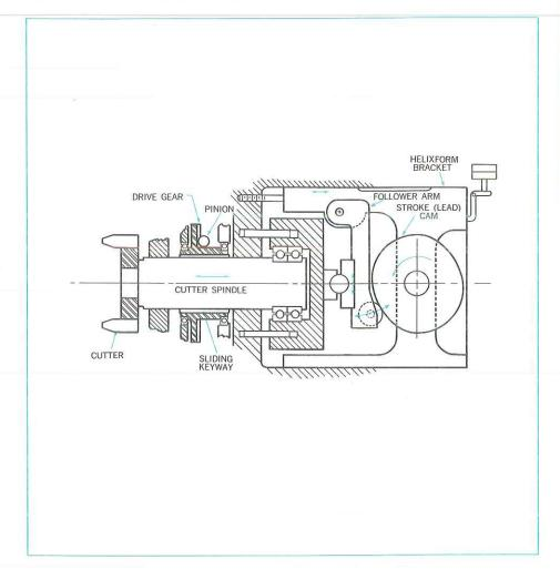
The diagram shows the cutter spindle, cutter drive gears and Helixform stroke cam mechanism. The cutter is driven by a pair of high reduction hypoid gears. The gear hub is rigidly mounted and restrained from axial motion in the cutter spindle
