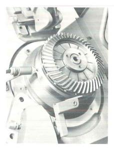
An optional deburring unit which is mounted on the workhead (as shown above) provides a quick and efficient means of removing the burr from the root of the finished tooth slot, thereby eliminating a separate deburring operation.
