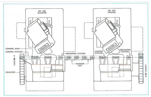
The Gleason No. 607 Hypoid Helixform Gear Finisher and its companion No. 606 Hypoid Gear Rougher can be equipped with a unique automatic loader and transfer unit, which has been designed and developed for low cost, large scale production.
