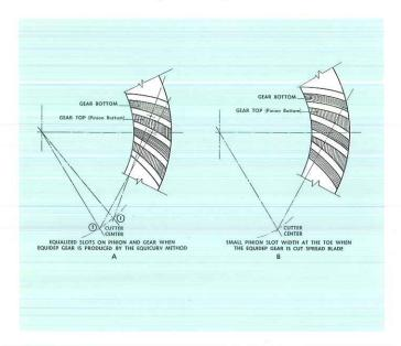
Figure A shows the equalized slots produced by the Equicurv Method. The taper is not removed but divided between the pinion and gear. The gear slot is tapered because the cutter center is at position 1 for cutting the convex side and at position 2 for the concave side. For an Equidep gear cut spread blade as shown in Figure B, the same cutter position is used for both sides.
